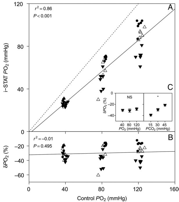
**Figure 2:** (A) Bar-headed goose whole blood  $PO_2$  measured with the i-STAT system vs.  $PO_2$  measured with a thermostated electrode (control) at 15 (inverted filled triangles), 30 (upright open triangles) and 45 mmHg  $PCO_2$  (filled circles). (B) The relative error of i-STAT  $PO_2$  measurements,  $\delta PO_2$  vs. control  $PO_2$ . (C) Effects of  $PO_2$  and  $PCO_2$  on  $\delta PO_2$ . See legend to Fig. 1 for further information.
