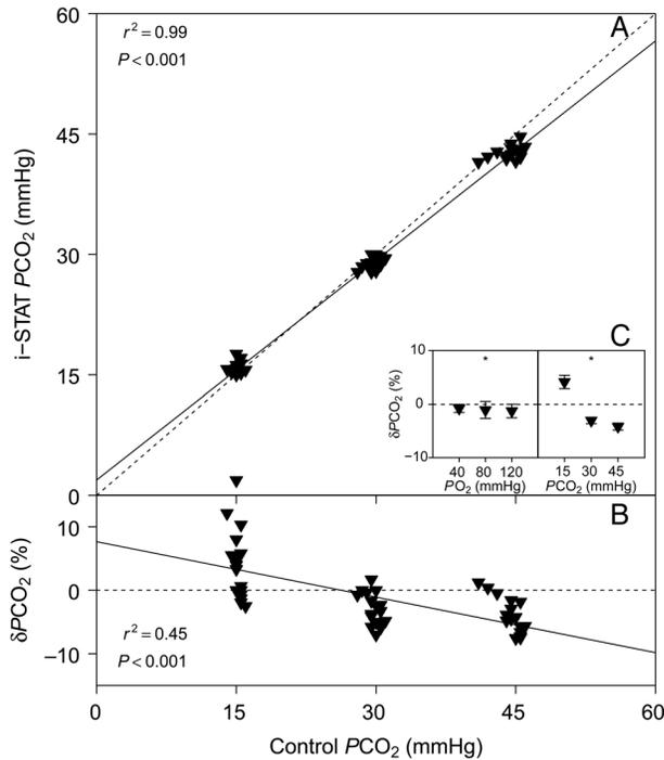
**Figure 4:** (A) Bar-headed goose whole blood  $PCO_2$  measured with the i-STAT system vs.  $PCO_2$  measured with a thermostated electrode (control). (B) The relative error of i-STAT  $PCO_2$  measurements,  $\delta PCO_2$  vs. control  $PCO_2$ . (C) Effects of  $PO_2$  and  $PCO_2$  on  $\delta PCO_2$ . See legend to Fig. 1 for further information.
